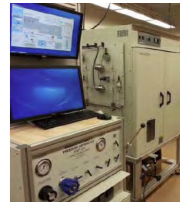
Core flood +MMP dual system
